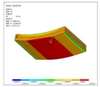
Fig.8 Transverse stress of A-Deck after reinforcement under consolidation constraint
