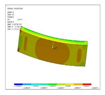
*Fig.5 Transverse stress of the A-Deck before strengthening under hinged constraint*
