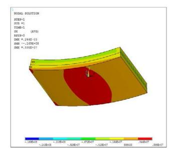
Fig.7 Transverse stress of A-Deck after reinforcement under hinged constraint
